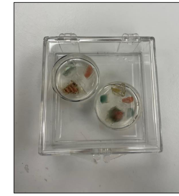
Figure 5: Separates in epoxy after polishing ready for laser ablation.
