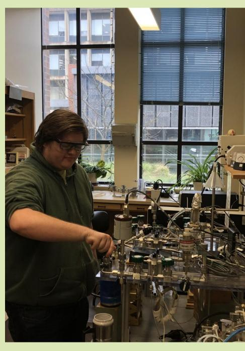
To get the desired result we had to use the mechanism at University of Oregon that would allow the delta 18 oxygen to be the only element that gets recorded. To achieve this, we had to turn multiple valves to release unwanted elements and freeze certain tubes to hold certain elements in place. As of a result the spectrometer was able to output the necessary delta 18 oxygen we needed.
